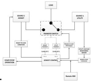
\* A utility voltage monitoring sensor (as shown in the AMF diagram above) must be connected in order to use the AMF feature on the 1302 control. Use Schneider Electric Relay RSB1A120U7 and Socket RSZE1S35M.
